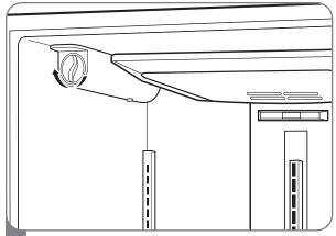
Use the handle to twist the cartridge clockwise about one turn, until the handle is in a horizontal position. You will feel the filter click into place.
