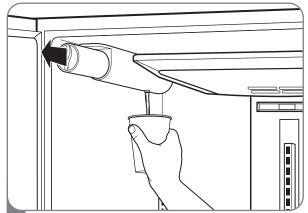
Remove the old cartridge. Take the new cartridge out of its packaging, and remove the protective cover from the o-rings. Hold the cartridge handle in its vertical position, and firmly push the new filter cartridge into place until it stops.
