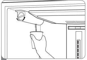
Rotate the knob of the old cartridge counterclockwise. When the cartridge is released, you will feel it click out of place.
