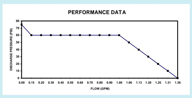
PERFORMANCE MEASURED WITH FLOODED INLET (0 PSI), 70°F (21°C) AMBIENT AND WATER TEMPERATURE, AND VOLTAGE CONTROLLED AT 115 VAC. FLOWS WERE RECORDED AFTER TEMPERATURES HAD STABILIZED. POSITIVE INLET PRESSURE WILL INCREASE THE MAXIMUM FLOW AT THE REGULATED DISCHARGE PRESSURE. MAXIMUM INLET PRESSURE IS 60 PSI.
