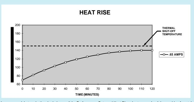
This pump model stays in the shaded area of the Performance Data and Heat Rise charts, meaning it is capable of sustaining continual running, at any of the above listed pressures, without shutting down to allow the motor to cool. To conserve wearing parts, however, the pump should only operate as needed.
