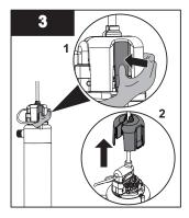
Remove the safety cap by squeezing the tabs.
