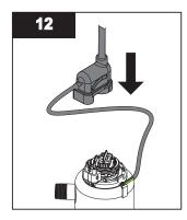
Align connections by rotating the ring clamp and install the lamp plug.
