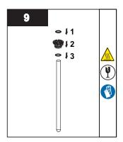
• Insert new O-rings and tighten the sleeve bolt to the quartz sleeve.
