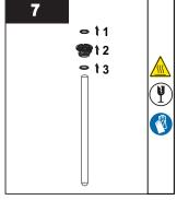
Unscrew the sleeve bolt and remove O-rings from the quartz sleeve.
