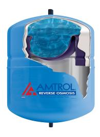
Polypropylene liner and butyl rubber diaphragm are locked together with Amtrol's unique hoop ring and groove design.
