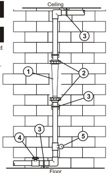
**3.** Wall, floor and ceiling mounts and supports are to be carefully aligned and sturdy. Wall, floor and ceiling supports are recommended as needed. This is to maintain pipe alignment and to prevent vibration.
