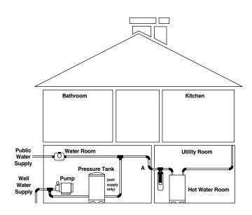
Your new **AP430** Hot Water Protection System installs on the cold water feed line before entering the water heater or boiler. Complete installation instructions included for your convenience.
