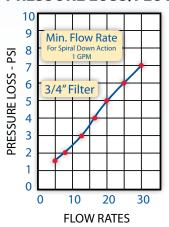
3/4" FNPT inlet and outlet 1/2" MNPT drain port Min. Flow Rate 1 GPM Max. Flow Rate 25 GPM
