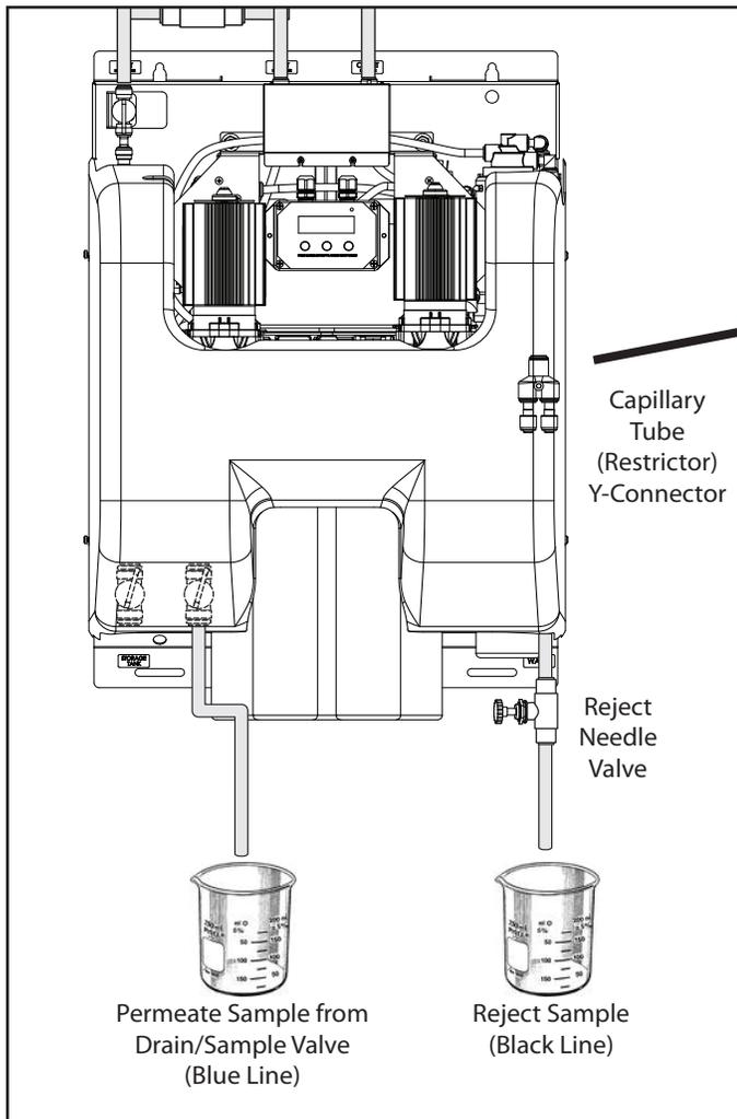
**Figure 6.** Capillary Tube (Restrictor) Y-Connector Detail
