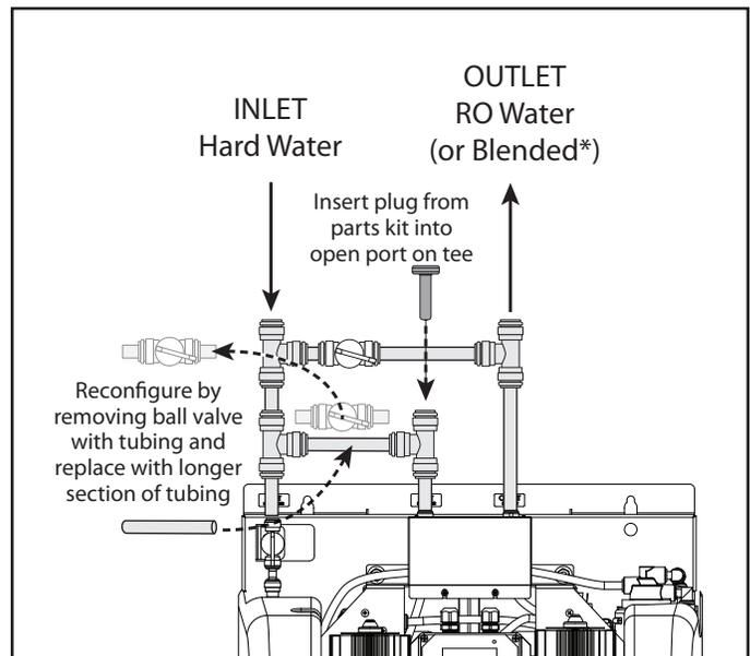
**Figure 4.** Reject Y-Connector Detail
