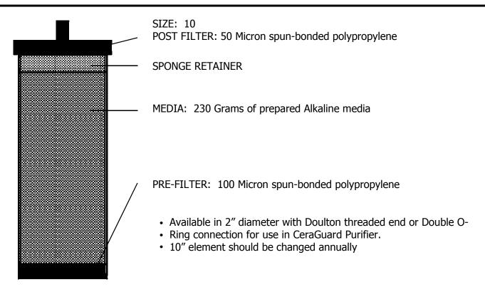
This element has shown to provide a pH balanced water of between 9.5 and 10 in case studies with an ORP potential that rivals ionizing machines.
