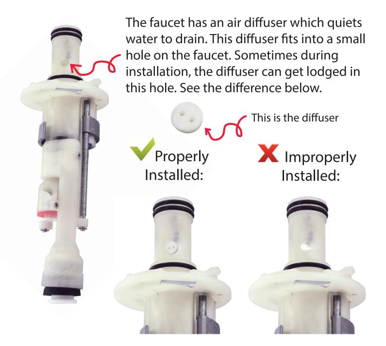
If the diffuser is not properly installed, the air disperser will allow a loud "gurgle" noise to be created when the RO is making water. Customer needs to check and verify white diffuser is present and is installed correctly.
