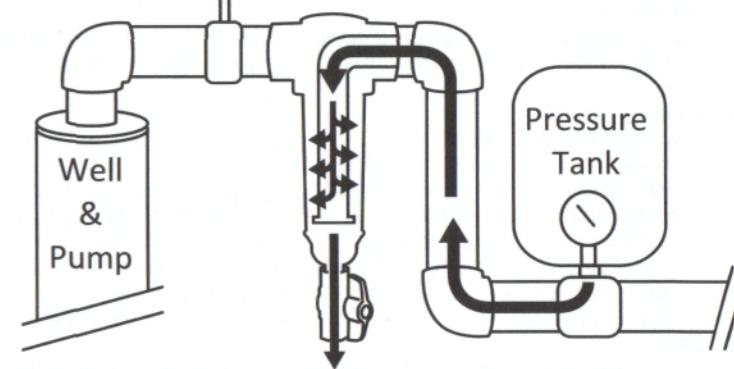
Install your SpinDown™ Filter before your pressure tank (and after the pressure switch) to enable clean water backflushing. Open the **purge valve** and water from the pressure tank will purge the filter from the inside-out.
