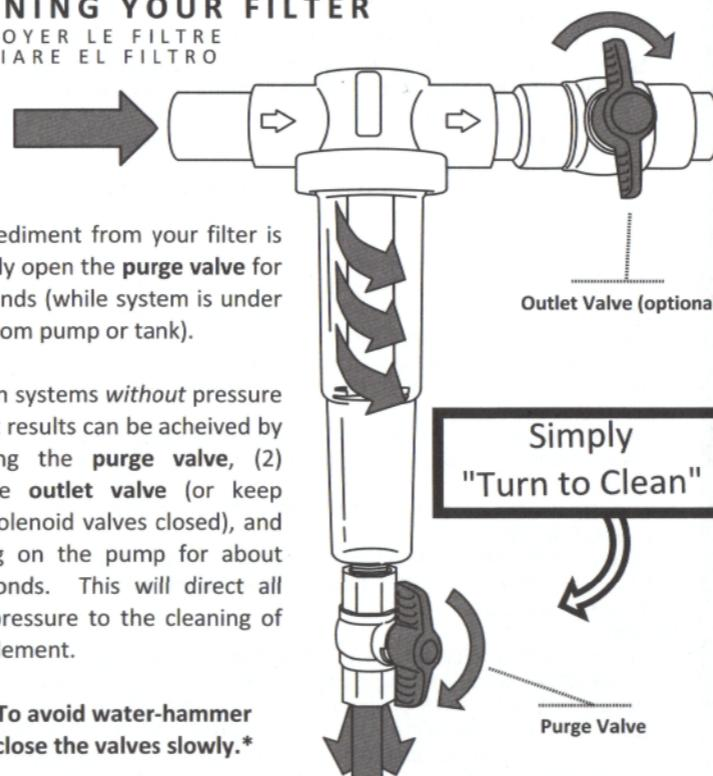
Cleaning sediment from your filter is easy. Simply open the **purge valve** for a few seconds (while system is under pressure from pump or tank).
