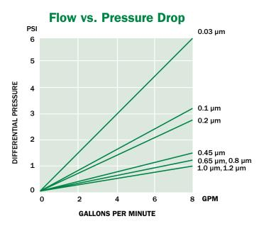
This chart represents the typical water flow per 10" cartridge length. Cartridges are tested in water at ambient temperature. Data may be extrapolated for multiple lengths, but as flow rate increases,  $\Delta P$  of the housing becomes more apparent.
