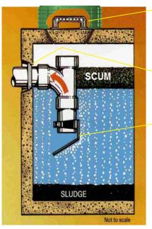
Concrete Lid Handle HDPE handle for precast concrete septic tank lid. Rated 500 lbs. Hand-lift only.
