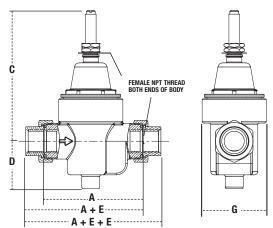
ABOVE VALVE SHOWN WITH SINGLE NPT UNION CONNECTION ON INLET VALVES MAY BE ORDERED WITH 0,1,0R 2 UNION CONNECTIONS USING ANY COMBINATION OF NPT, SOLDER, PEX OR CPVC CONNECTIONS REQUIRED
