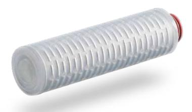
HP-PP Series filter cartridges are absolute rated, pleated depth-type filters, constructed of 100% polypropylene material. These filters are available in absolute particle retention ratings from 0.1 to 5 micron and various end cap configurations to fit into the most standard housings. All components of the HP PP series filter cartridges are FDA approved.
