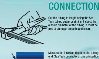
Measure the insertion depth on the tubing end. Sea Tech connectors have a insertion depth line molded onto the outside of the connector bodies.
