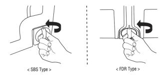
Turn on man water supply valve to the refrigerator first. Run water through the dispenser for 6 minutes (3 gal) to purge the system
