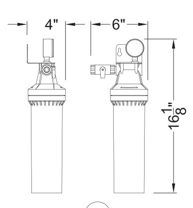
System Tested and Certified by NSF International against NSF/ANSI Standard 42 Aesthetic Effects - Particulate Reduction (Class I) and the reduction of Chlorine, Taste and Odor.
