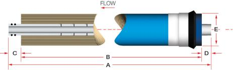
All TF - 1812 Residential Membrane Elements seal at a standard 2.00 inch - 2.05 inch I.D. within membrane housings.
