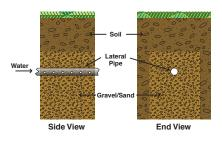
Water flows out of the laterals into a bed of gravel or sand which acts as a final filter before the water enters the ground.
