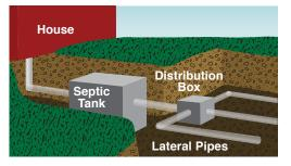
Septic tanks are designed to allow bacteria and enzymes to biodegrade organic waste. This amazing process actually converts waste into water, carbon dioxide, and small amounts of mineral matter!
