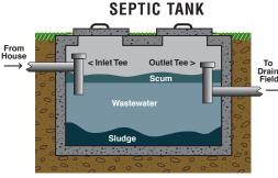
Incoming solid matter sinks. Soap and grease float. The tank has an outlet baffle to hold in undigested waste. Only clean water should leave the tank and enter the lateral pipes.
