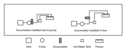
It is recommended the pre-charge be checked annually or anytime the accumulator does not appear to be functioning properly. Temperature and altitude changes can affect the accumulator pressure and performance. Use any standard tire pressure gauge to check pressure.
