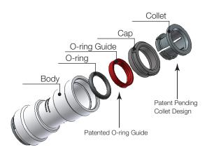
AquaLock<sup>™</sup> incorporates an exclusive O-ring guide for improved reliability. This unique feature ensures zero-leak connections by:
