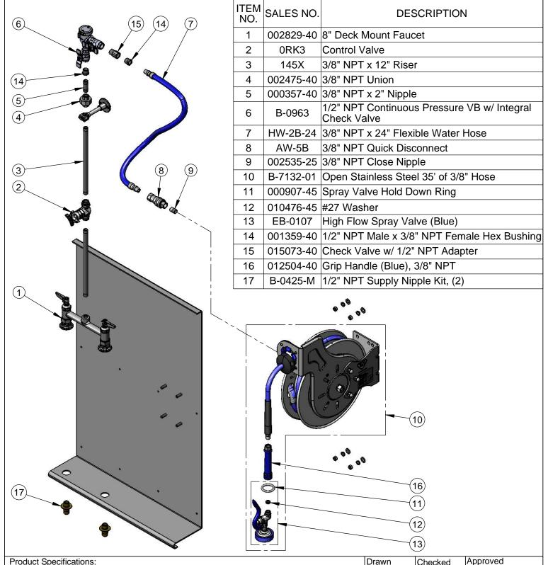
Open Stainless Steel Hose Reel w/ 35' of 3/8" Hose on Stainless Steel Backplate, High Flow Spray Valve (Blue), Vacuum Breaker, 3/8" NPT Flexible Water Connector, 8" Deck Mount Mixing Faucet, & Control Valve
