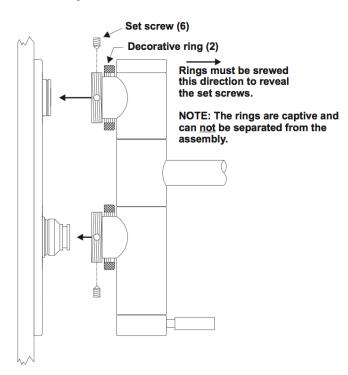
**Important note:** If the set screw points are not properly seated into the "V" groove, the tops of the set screws will not allow the decorative rings to be threaded into place — **this is a safety feature that assures a proper connection to the pipe adapter.**
