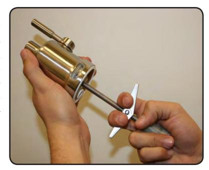
Disassembling your faucet is never recommended as this could void your warranty. If it is necessary to remove the fitting at the end of the toggle bolt you must follow the following procedure for re-assembly. Prior to re-connecting the fitting to the toggle bolt, you must insert the 3/8" blue tube into the fitting. There are small O-rings inside of the fitting that could be pushed out of position if the blue tube is not fully inserted first. Failure to do so may cause the faucet to leak.
