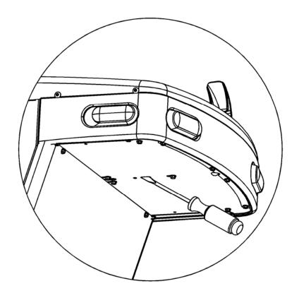
To adjust stream height, insert a 1/8" Flat blade screwdriver into the slotted hole as shown. The screwdriver will engage the stream height adjuster in the cartridge plunger. Turn clockwise to increase stream height, or ccw to reduce stream height.
