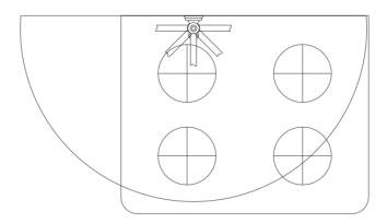
mounting plate to secure to the wall, some play between 1/8" and 1/4" will make the alignment easier). The height of the stub out pipe should be approximately 15 inches above the cooking surface. This will allow adequate clearance for most larger cook pots that will be filled by your potfiller. (see diagram below for behind the wall installation)
