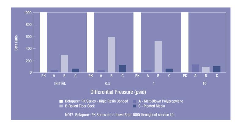
As illustrated in Graph 1, the performance of the Rolled Fiber Sock cartridges (Competitor B) exhibits contaminant unloading and a loss of filtration efficiency as differential pressure increases from 1 to 10 psid. The Melt-Blown (Competitor A) and the Pleated Cellulose/Polyolefin (Competitor C) filters exhibit minimal contaminant retention through the test duration.
