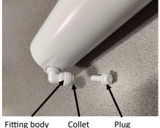
**2.** Remove the plug from the drain outlet fitting by pressing the collet towards the fitting body while pulling the plug out
