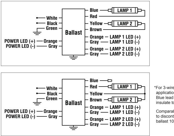
\*For 3-wire output application, cap Blue lead and insulate to 600v.
