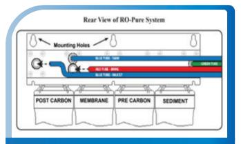
Remove the old RO membrane from the third head on the manifold
