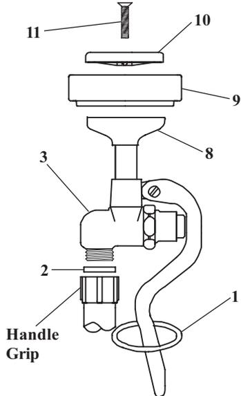
8. To replace no.2, unscrew *handle grip* from no.3 and replace with new no.2.
