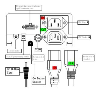
The various input and output connections for the SIP 2000 are conveniently located on the bottom of the main control unit. For operation, insert the female end of power cord A into the male Plug A (shown in diagram above with a red "in" label) The opposite end of Plug A will fit a standard wall outlet but should not be plugged into a power supply until the SIP 2000 has been completely installed in the water dispenser.
