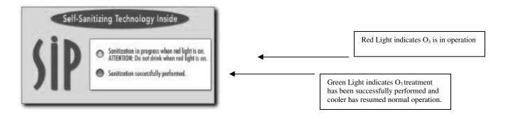
The external indicator light is only used to display the working status of the various functions when the SIP2000 machine is in normal operation. This optional led feature can be fitted to the front of the water cooler and mounted on the label provided.
