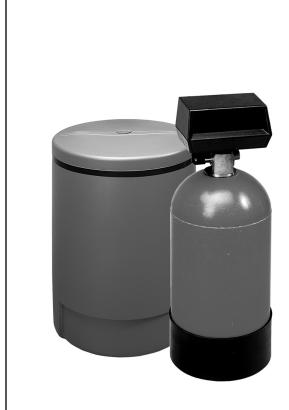
HWS050 Rated for 16,000 grains per tank, 5 gpm (18.9 lpm) service flow, 150°F (65.6°C) application:
