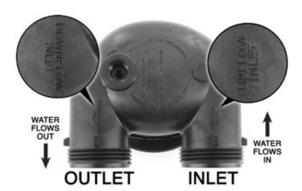
NOTE: This is a UPFLOW filtration system and is fed through the UPFLOW INLET. Feeding he system from the downflow inlet will cause the system to not filter properly
