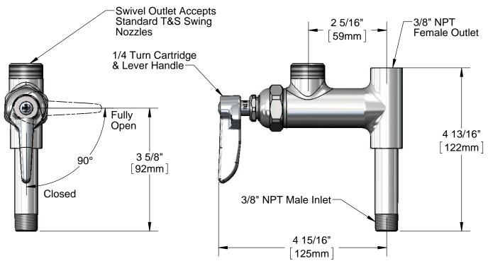
Add-On Faucet is an Addition to Pre-Rinse Units and is Installed in Outlets of Base Mixing Faucets of Units Before Fitting Riser Pipes.
