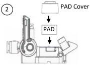
Place an absorptive PAD in the cup and put the PAD cover down over the top of the PAD. 3
