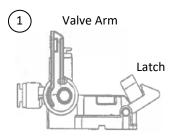
Move the latch to release the valve arm to the up, valve closed position.
