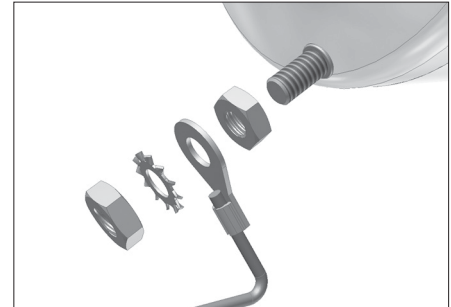
Step 1 – Disconnect Power to Water Purifier and Remove Ground Connector
