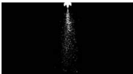
Straight through design squeezes fluid flow to create the spray pattern versus deflecting fluid flow and creating un-needed spray drift.
