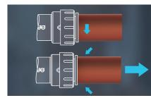
Depressurize the system. Turn locking cap quarter turn counter clockwise. Depress collet against the fitting and remove pipe.
