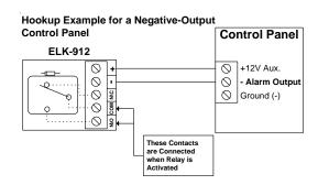
**Example 2:** If control has a negative output, connect the "+" terminal of the ELK-912 to the control's +12V terminal. Connect the "-" terminal of the ELK-912 to the negative alarm output.
