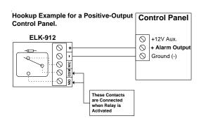
**Example 1:** If control has a positive output, connect the "-" terminal of the ELK-912 to the control's ground terminal. Connect the "+" terminal of the ELK-912 to the positive alarm output.
