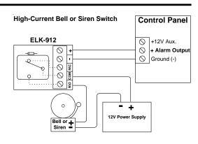
**Example 4:** ELK-912 used to switch a high-current siren or bell from separate power supply.
