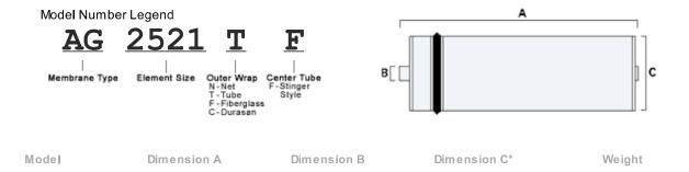
AG2521TF 21" (533 mm) 0.75" (19 mm) 2.40" (61 mm) 1.3 lbs (0.6 kg) \*The element diameter (dimension C) is designed for optimum performance in Osmonics pressure Vessels. Other pressure vessel dimension and tolerance may result in excessive bypass and loss of capacity.
