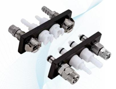
**Multi-Mount couplings** provide one easy-to-use coupling for connecting from three to five lines at once. Multi-mount couplings are available in a wide variety of materials including acetal and chrome-plated brass. Multi-mounts are keyed to prevent mismatched connections and can be configured with or without valves for maximum design flexibility.
