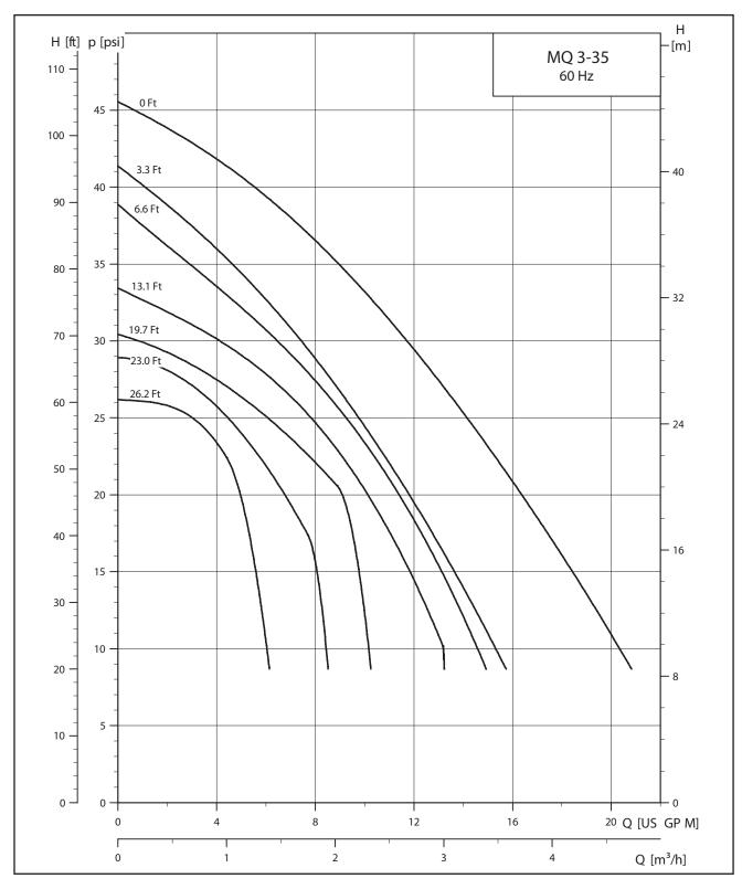
Provided it is filled with water, the pump is able to lift water from a depth of 26 ft (8 m) in less than 5 minutes.
