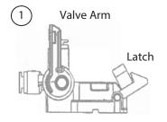
Move the latch to release the valve arm to the up, valve closed position.
