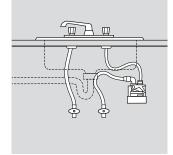
Mount filter head and connect water supply to inlet of filter head.
