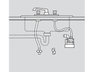
Shut cold water supply off and disconnect cold water hose.
