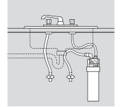
Install vertically with cartridge hanging down
