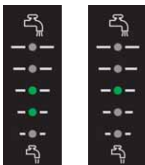
Fig. 15 SCALA2 outlet pressure indication
