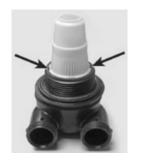
Screw the head on to the tank. Fit the basket over the distributor. tube and push down to get the threads to line up. Tighten until it's snug, no tools are necessary. Be sure and remove the tape from the end of the distributor tube first!!
