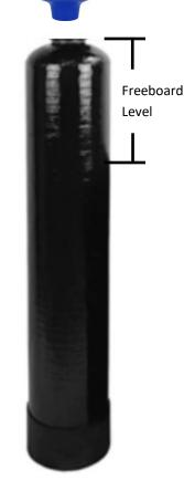
Be careful to not overfill the tank with media. Also important to have adequate freeboard space so media can expand during service flow. Overfilling can cause media to escape tank and get into house hold plumbing
