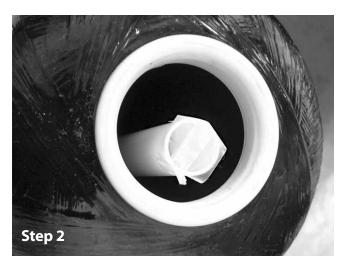
**Step 3**Place funnel into fiberglass tank, fitting the tube into the middle of the funnel.
