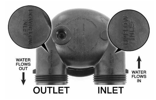
NOTE: This is an UPFLOW filtration system and is fed through the UPFLOW INLET. Feeding the downflow inlet will cause the system to NOT perform to specifications.
