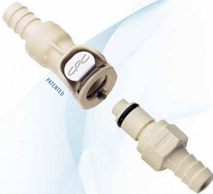
The 1/4" flow polypropylene PLC12 offers many of the same configuration options as the PLC. The polypropylene material adds greater chemical resistance for more demanding applications. PLC12 couplings are also gamma sterilizable. PLC12 couplings are also gamma sterilizable and available with optional RFID (Radio Frequency Identification) capability (see page 96).
