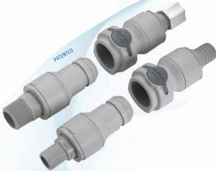
**NSH Series couplings** couplings are general purpose versions of our pressure-balanced, non-spill, ChemQuik® CQG06 couplings. Molded polypropylene, EPDM seals and a 100% springless and metal-free flow path provide broad chemical resistance and exceptionally high flow capacity, allowing instant disconnects (and reconnects), even under pressure. Their non-spill design virtually eliminates spills, minimizes downtime and enhances operator safety in a very low cost package.
