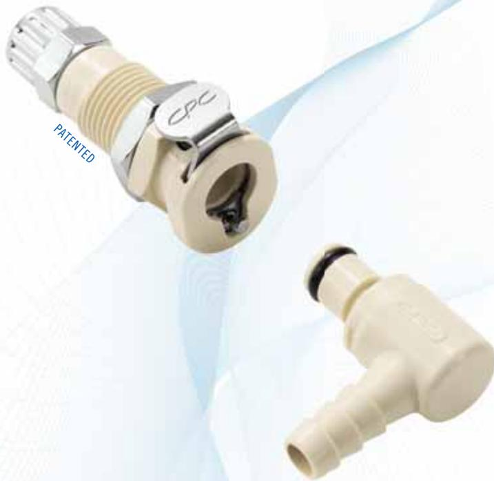
The 1/8" flow polypropylene PMC12 offers many of the same configuration options as the PMC. The polypropylene material adds greater chemical resistance and is gamma sterilizable. The PMC12 also mates to small diameter rigid tubing. Available with a 1/4-28 flat bottom port and 1/4-28 UNF threads, these couplings eliminate the need to thread and re-thread common compression nuts each time a tubing connection is made.
