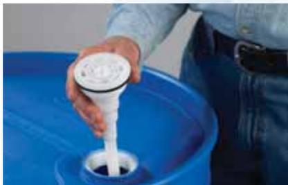
2 Place the drum insert assembly in drum.
