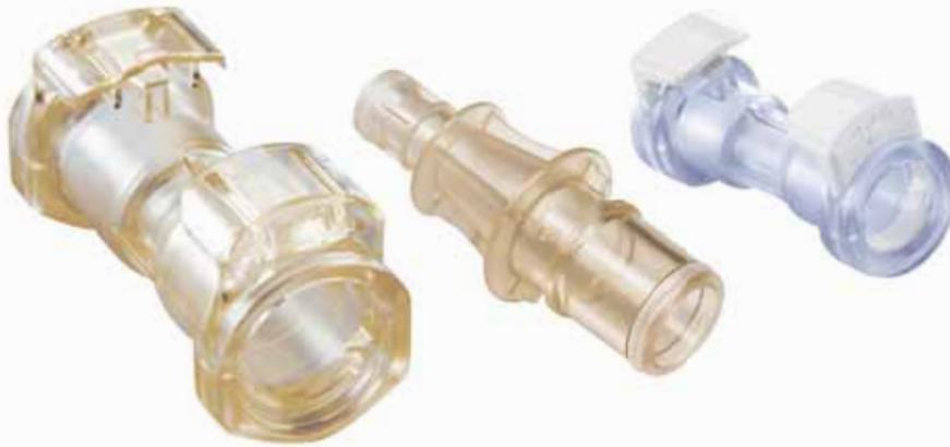
**MPC/MPX Back-to-Back Adapters** give end users the flexibility of connecting single-use systems that feature identical coupling connections at the end of their tubing. Combining both MPC and MPX couplings provides a reducing option for users who need to transition between tubing diameters ranging from 1/8" to 1/2".
